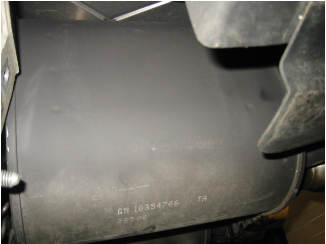
Grind smooth, painted and installed
